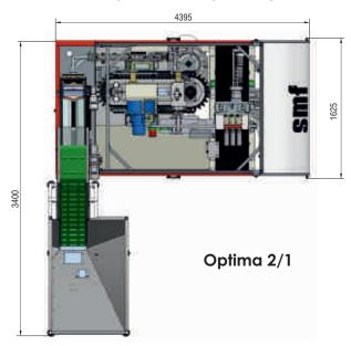
in upright position. With 6 cavities version, it is possible to produce bottles up to 3L, with nominal working speed 10000 bph of 1l. suitable for bottle 200 ml-3000 ml. **Optima 4MAX** is 4 cavities machine with nominal working speed 7000 of 1L, suitable for bottles up to 6000 ml. **Optima** machines are designed for customers interested in high advanced and reliable blower.
