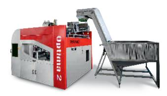
**Optima MAX** are special versions of classic 8 cavities machine with all advantages of **Optima** series - reliable operation and easy use - central lubrication system, pyrometers, quick mould-change system, detection of cracked bottles, router for internet connection, preform dumper. This modern machine is fully electric with all vital processes controlled and steered by Mitsubishi servo drives and ready bottles are discharged
