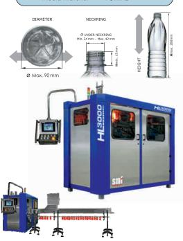
HL 3000 and CL 200 / 400 are fully automatic linear PET blowing machines suitable for production of bottles 200 ml - 2000 ml.
